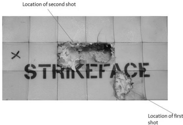
Figure 1: Ceramic Armor after Ballistic Testing
